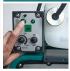
The DoseMatic<sup>®</sup> kit (optional) allows real time adjustment of the percentage of detergent being delivered to the floor, for optimum results, without waste.
