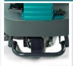
The traction motor is sealed and protected by a robust steel bumper which also incorporates an anti-tilt device. The tyre of the drive wheel is made of non-marking and anti-skid polyurethane.
